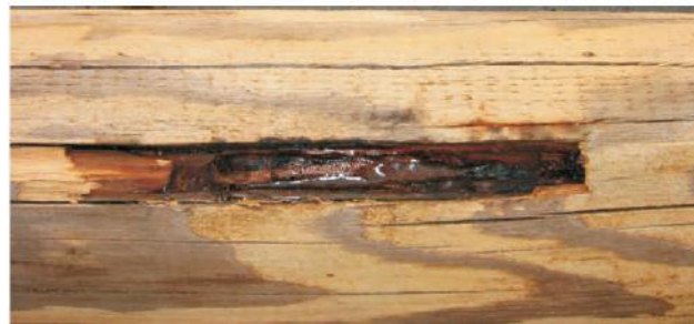
Wood fibers consolidated with M-Balm.
