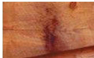
Dark colored streaks caused by metallic tannates. Oxcon solution will also remove rust stains caused by nails, screws and fasteners.
