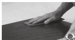
SANDING #120-#150 GRIT WITH THE GRAIN
